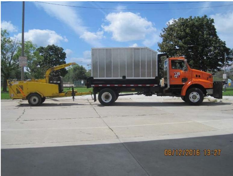
AFTER PICTURE 2016 #4 AS FALL LEAF BUNCHING TRUCK W/BALLAST LOAD OPTION
