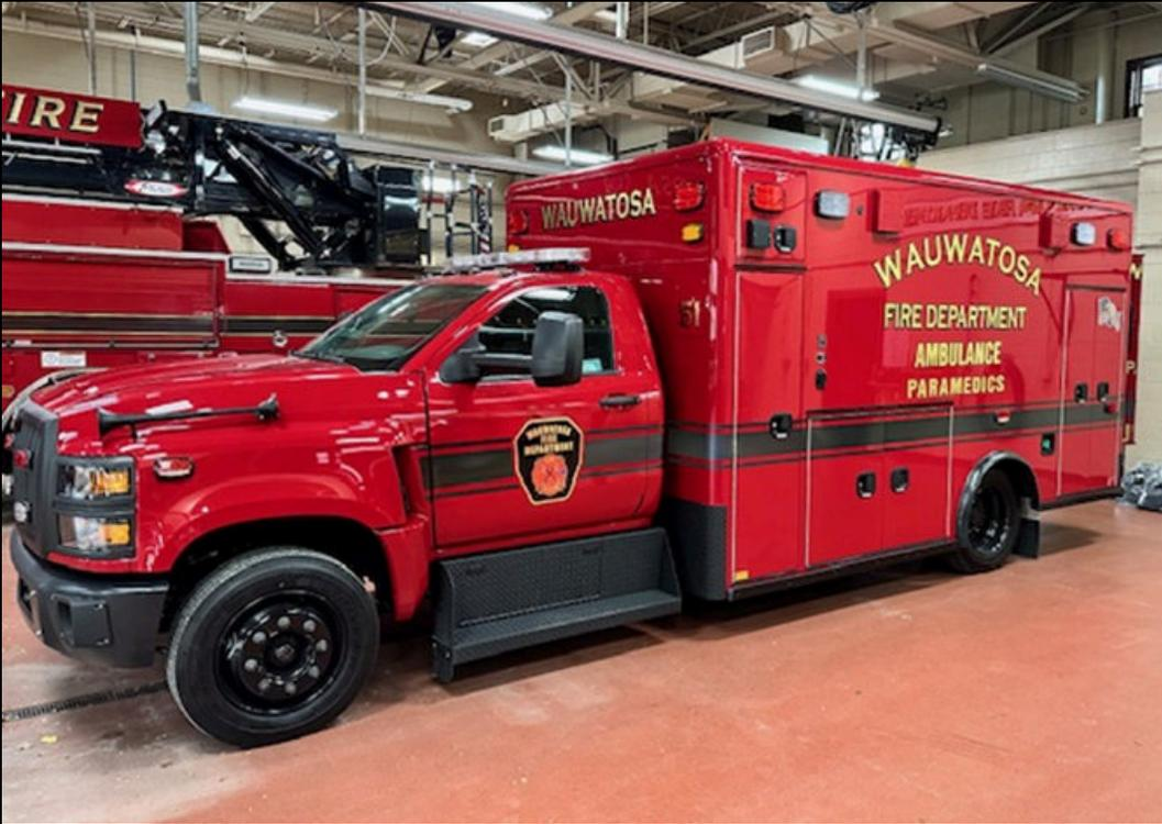
Med 51 was built in 2023 by Horton Emergency Vehicles. The chassis is a medium duty International CV 4x2 with liquid springs to assist in providing a smooth ride for the patients during transport to the hospital. This Paramedic ambulance is equipped to treat and transport patients to the hospital. In addition to extensive life-saving medical equipment, this ambulance also is equipped with firefighting equipment.
