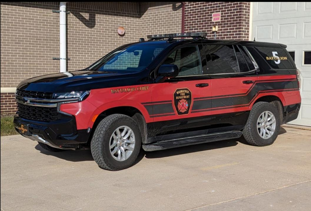
The function of Battalion 5 is to serve as the Battalion Chief on duty and respond to major incidents in and out of the city. This vehicle is a command center on wheels when significant incidents occur. It is a 2023 Chevy Tahoe with extensive radio communications equipment capabilities, a computer for mapping and messaging, rescue task force equipment, meters for hazardous situations and a self-contained breathing apparatus (SCBA) for fire scenes.
