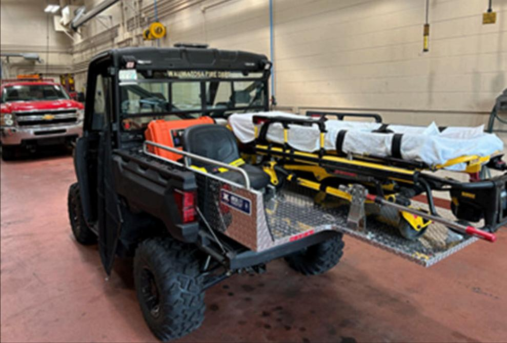
UTV 56 is a 2023 Polaris Ranger equipped with four-wheel drive, a winch, a cot, and medical equipment that was fully funded with grant money. The unit is available and appropriate for a wide variety of emergent and non-emergency uses, which may include, but are not limited to:
