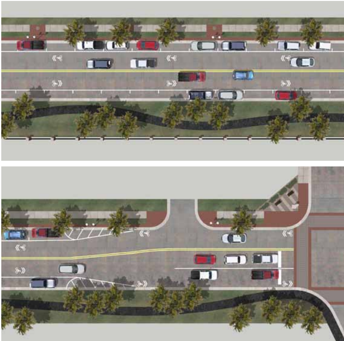
Figure 4.14: State Street Sections
