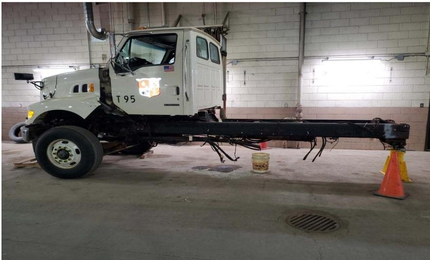
T-95 WILL BE RE-PURPOSED AS AN ANTI-ICING PLOW TRUCK, WITH THE ABILITY TO SPREAD 950 GALLONS OF SALT BRINE TO PRE-TREAT ROADWAYS PRIOR TO WINTER STORM EVENTS.
