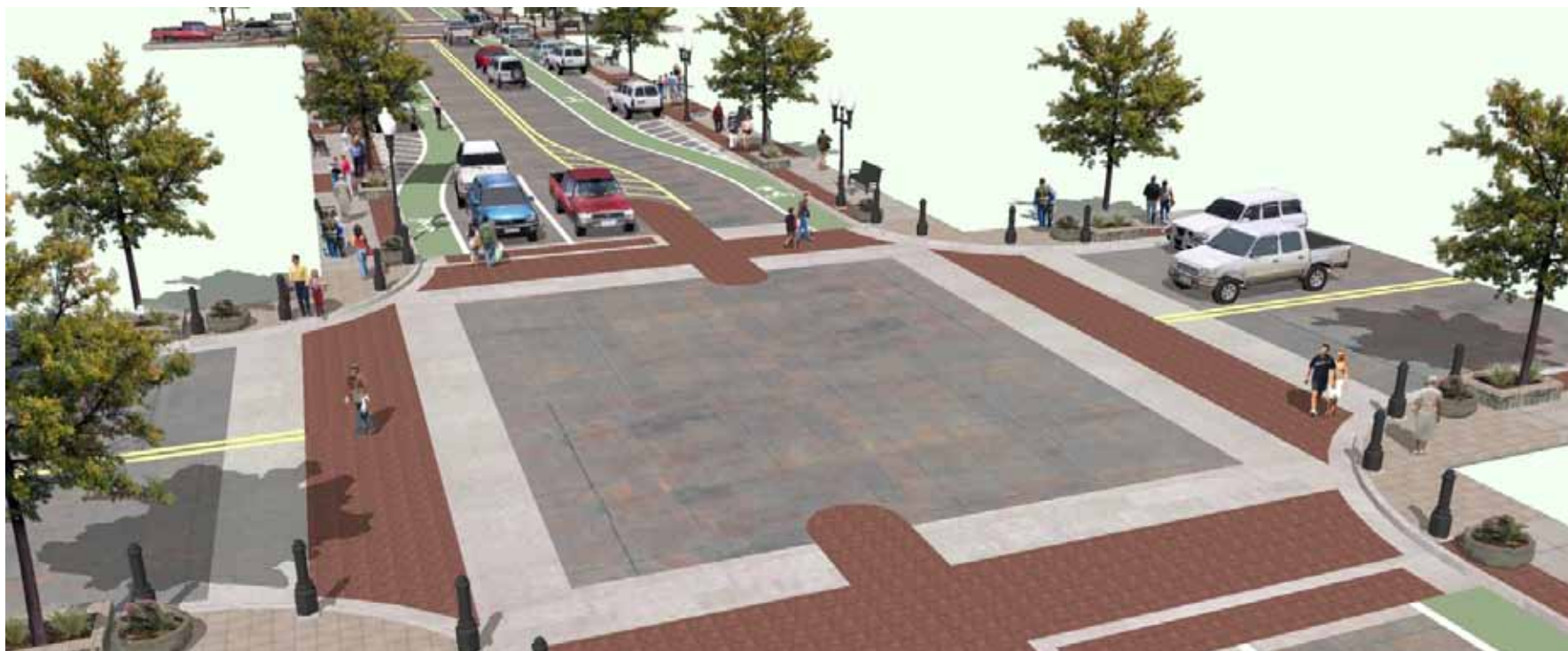
↓ North Avenue Plan View. Right-hand intersection, at 60th and 68th Streets, provides a protected left-turn lane and a surface median refuge for pedestrians. Left-hand intersection is typical, and includes a four-way stop at 64th and 72nd. ↑ North Avenue Perspective. View looks west from 60th or 68th Street intersection.
