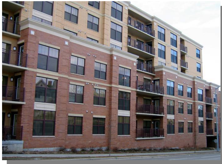
Example of how the human scale of a building can be enhanced by “stepping back” upper stories
